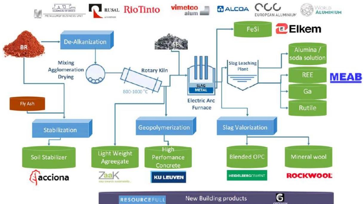
The figure demonstrate the production of REE concentrate, Ga concentrate, alumina/soda solution and rutile concentrate from the hydrometallurgical processing of engineered slags/sinters produced in RemovAL pyro-metallurgical pilot plants. Ga is co-extracted both from the slag and the Bayer liquor. At least 500 kg of slag and 100 l of Bayer liquor will be processed at **MEAB** solvent extraction pilot plant in Germany.
