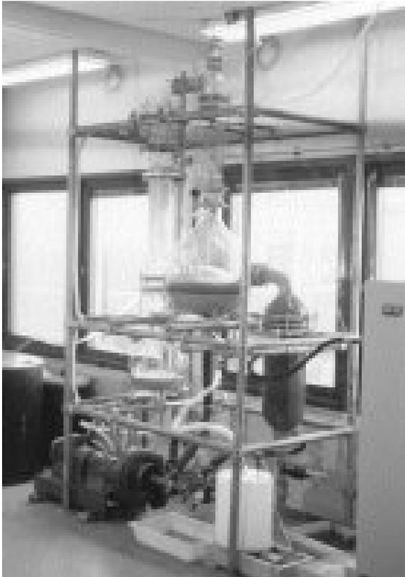
**Cadmium Carbonate Precipitation Equipment**
