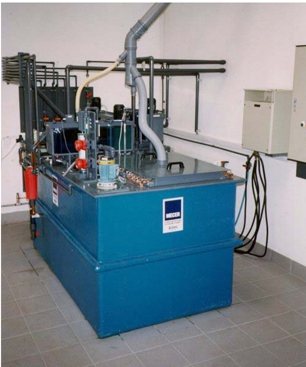
MECER Recovery Unit Integrated in the Production of Printed Circuit Boards
