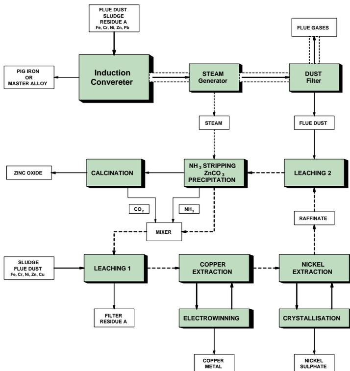
The feasibility of a pyro/hydro-metallurgical UDDAMAR process as a centrally located recovery plant for the treatment of oxidic and hydroxidic metal containing waste from steel and metal works, including the plating industry, has been investigated some years ago in Sweden. The process, shown in the figure, is based on the use of the UDDACON induction converter and the AmMAR wet process technology
